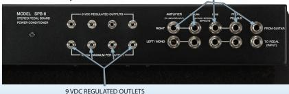
9 VDC REGULATED OUTLETS FOR PEDALS, 100mA MAXIMUM PER OUTPUT
