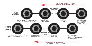
Note that there are two seperate channels, **LEFT** (mono) and **RIGHT** (stereo). If nothing is plugged into the effects return jack, the signal will flow unimpeded from the first jack, **IN FROM PEDALS**, to the **OUT TO AMP INPUT** jack. The send jacks are unswitched and may be used to take a "tap" off the signal path without breaking it, provided the effect return jack is not being used.
